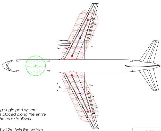
Denotes coverage when using single pad system. The single pad system can be placed along the entire length of the fuselage or on the rear stabilisers.
